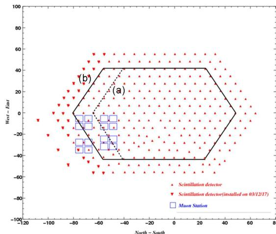
Fig. 1. The GRAPES-3 air shower array; The detectors in the regions bounded by the solid line and dotted line are the trigger detectors.
