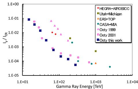
Fig. 2. Upper limit of the ratio of isotropic gamma rays to cosmic rays. The results of the HEGRA-AIROBICC [11], Utah-Michigan [12], EAS-TOP [13] and CASA-MIA [14] experiments and previous (1999 [8], 2001 [9]) and this work with the GRAPES-3 experiment are shown by the points, as indicated in the legend.
