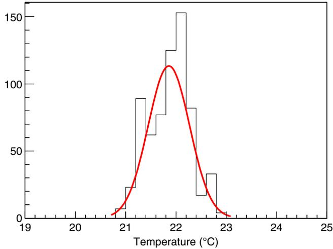
**Figure 3.** Temperature distribution inside the muon supermodule. Gaussian fit yields  $\sigma = 0.4^{\circ}\text{C}$ .
