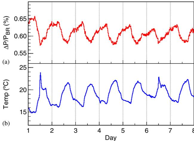
**Figure 2.** Variation of (a) fractional pressure  $\Delta P/P_{BR}$  and (b) temperature  $T$  in the control room over a period of one week.
