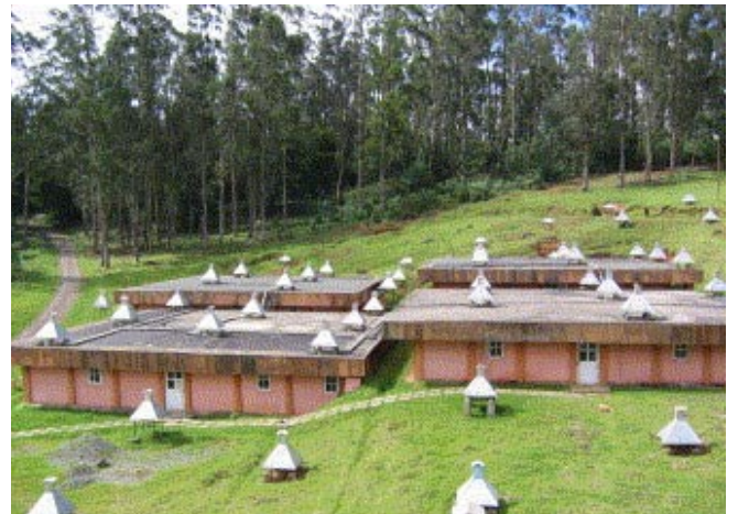
FIG. 2 (color online). A view of the GRAPES-3 experiment showing the four halls housing the four supermodules of the muon detector. The scintillator detectors of the GRAPES-3 air shower array, placed on the roof and around the muon halls are also visible.
