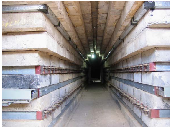
Fig. 3. An inside view of a super-module showing the proportional counters and layers of concrete blocks for two of the four modules. The remaining two modules are located further inside.
