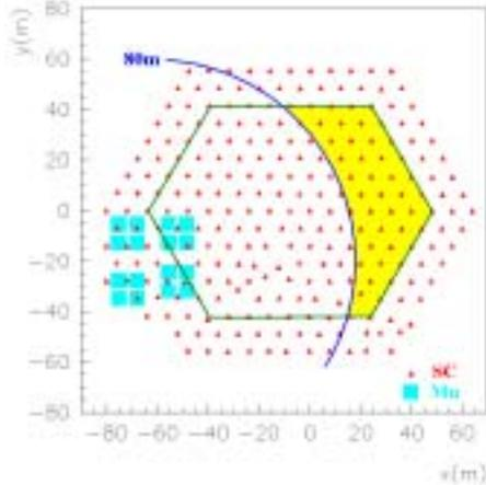
**Fig. 1.** Accepted core location. Triangle marks mean SD arrangement and square ones mean muon detectors. For this analysis, core location should be in yellow (or gray) area, which is inside a hexagon and  $80m$  away from muon detectors.
