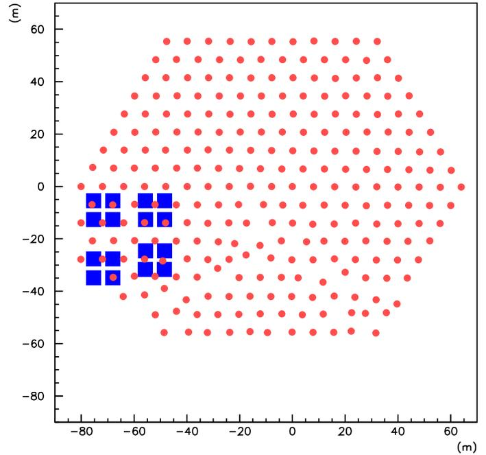
**Fig. 1.** A schematic layout the GRAPES-3 air shower array shown here with 217 detectors (circles). Each of the 16 squares represent a 35 m<sup>2</sup> area tracking muon detector with  $E_{\mu} \geq 1$  GeV used in the present work.
