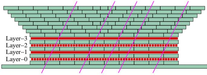
**Fig. 2.** A schematic display of the 4-layer tracking muon telescope module with 58 PRCs per layer. The four layers of the PRCs labelled Layer-0, Layer-1, etc. are embedded in concrete blocks. Inclined lines represent a set of parallel muon tracks.
