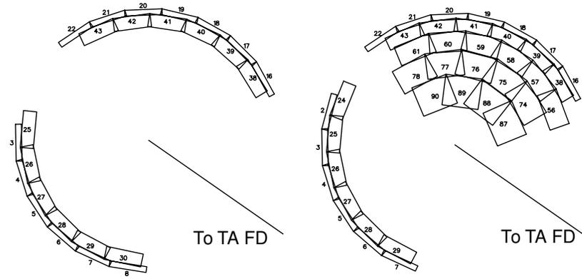
**Figure 3.** Arrangement of HiRes mirrors at 6 km, in the center of view of the TA FD sites. The individual mirrors are seen in top-projection view, covering elevation angles from 3 – 31°. The site on the right also shows the 15 tower mirrors placed to view higher elevations
