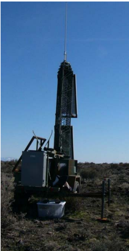
Figure 4. The communication tower. This is the tower setting temporarily. We will construct communication towers fixed ground. These are 15m heights and have the lift of directional antennas. Communication towers will set 5 places and they will be able to communicate each other.
